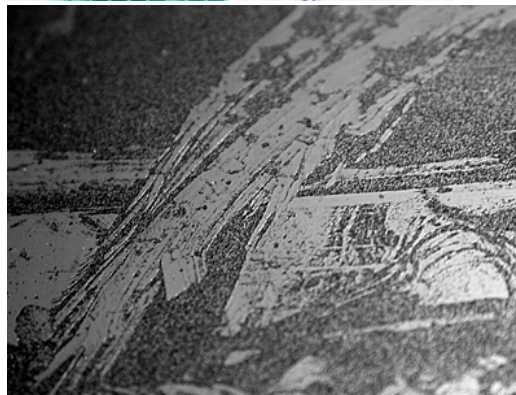
Plastic grill in mordant tray keeps plates off the bottom. Action of copper sulfate on crystalline structure of aluminum.
