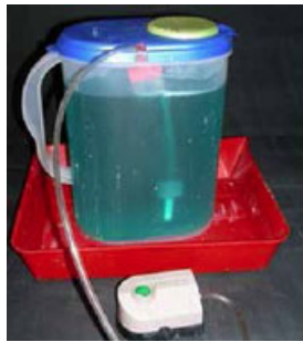
Simple vertical tank: For my research, I found that a vertical tank with air bubbling from the bottom is the best method of introducing oxygen to the solution and keep things circulating. A cheap aquarium pump can be left on all the time to regenerate the mordant.
