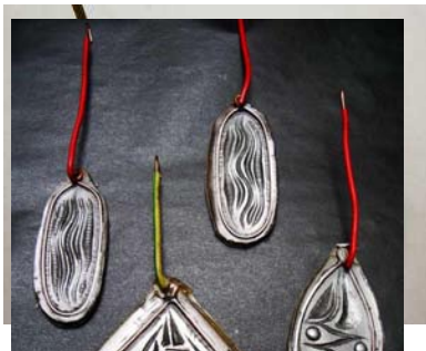
Left - wax mould ready to deposit copper by galvanizing finished pendant
