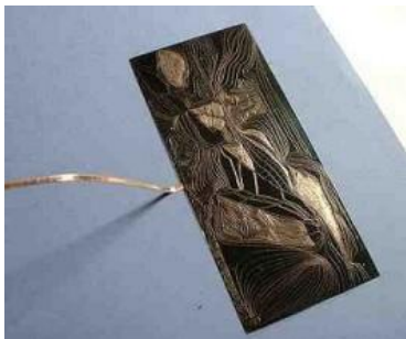
Below - strip bent up to project out of electrolyte.
