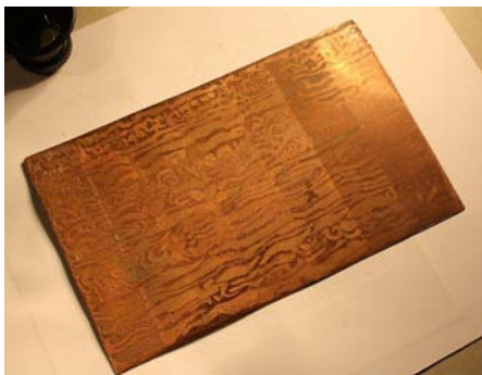
Above – small copper test plate after sugar lift tinting and stopping in 7 steps of about 15 minutes at 1 volt.
