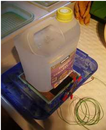
Weight on Galv-On sandwich - 5 litre can of water
