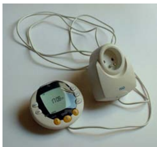
An electronic timer unit to control the mains electricity supply to the power supply unit (battery charger or other) with digital display and setting buttons on an extension lead.
