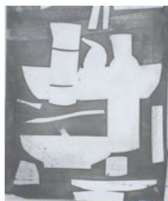
Zinc plate after electro-etching in sodium chloride electrolyte
