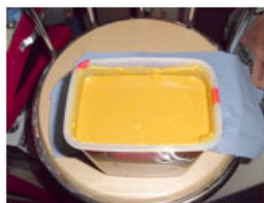
Yellow cuprous oxide produced in sodium chloride electrolyte after electro-etching a copper plate
