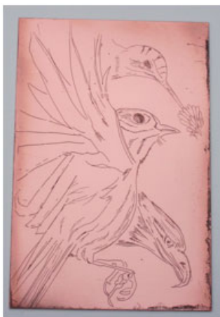
Copper plate after electro-etching in sodium chloride electrolyte
